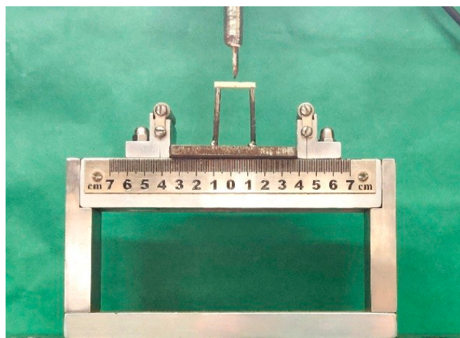
Figure 4. 3-point bending test in Universal Testing Machine
