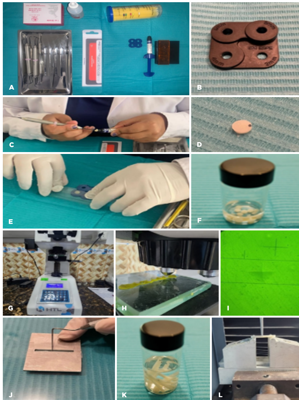
Figure 1. Experimental workflow: 3M mold for disc fabrication (A); composite placement with Hu-Friedy instrument (B); surface parallelization with matrix strip and glass slide (C); finished/polished disc (D); disc storage (E); Vickers microhardness testing (F); indent placement (G); indentation (H); mold for bar fabrication (I); bar fabrication (J); bar storage (K); three-point bending on universal testing machine (L).
